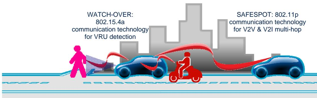
**Figure 5** An overview of the interconnections between the SAFESPOT and the WATCH-OVER Communication technologies
